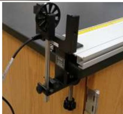
Pictures of the apparatus. The photogate, threaded rod, and pulley unassembled (top). The assembled photogate unit (bottom left). The Assembled photogate unit on the right angle clamp with track (bottom right).
